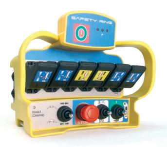
**GREEN LED ON** = the operator is inside the safety ring.
